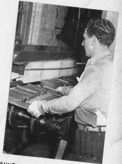
ANNEALING PLUMBING FITTINGS SO THEY'LL STAND PRESSURE AND LONG WEAR KEEPS ARMY VETERAN CARL D'ANDREA BUSY NOW.
