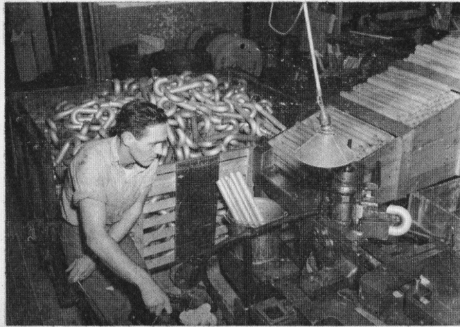
A HOME WITHOUT PLUMBING ISN'T MUCH GOOD. HERE NAVY VETERAN JOHNNY BAKER BENDS TUBES FOR TRAPS THAT WILL SOON BE IN NEW HOMES.
